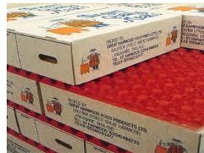
Freezer spacers play an important role in the frozen food and cold storage industry. These spacers are used to minimize product freeze time, saving on utility costs. With these spacers, cold air can move between layers of products resulting in consistent freezing for the entire pallet load. Once the products have reached a certain temperature, you can remove the spacers between stacks of products.
