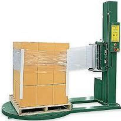
Stretch wrappers are pieces of equipment that provide an efficient way to unitize and secure pallet loads with plastic film. In the frozen food industry, stretch wrap also influences the rate at which food thaws and freezes, so choosing the best wrap for your industry and the best tool to help you wrap is especially important.
